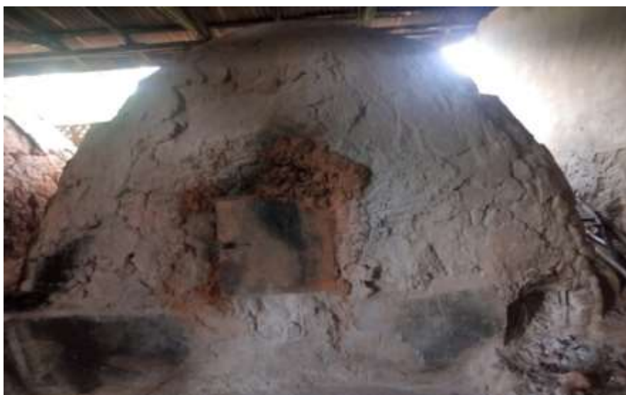
Plate 1: Burning of Sugarcane Fibre Ash in a Local Oven
